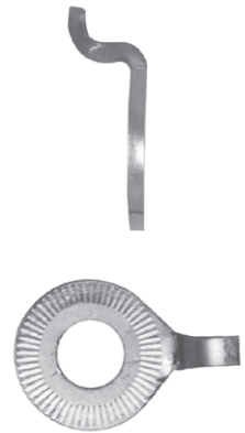
Special safety washer - must be mounted on all bikes with disc brakes, unless the fork has reversed fork ends
